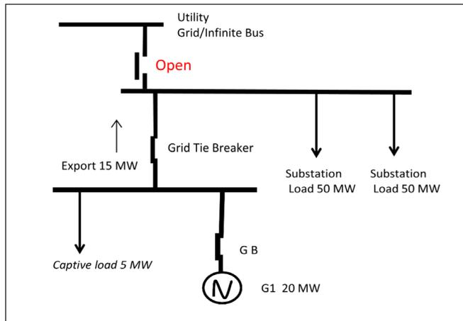
Fig. 5: Loss of grid/utility
