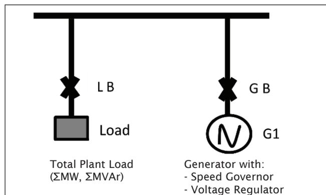
Fig. 1: Stand-alone mode of generator
