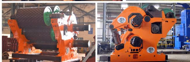
efficiency and performance of the Ulka CMR mills. This is complemented by the fact that, at the same time, power consumption is reduced by about 1.0 kWh per TCH per mill, as compared to the conventional six-roller mill.
