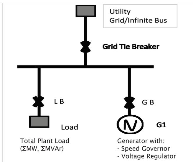
Fig. 3: Generator paralleled with utility grid
