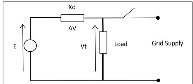
Fig. 6: Equivalent circuit of the synchronous generator operating parallel with the grid
