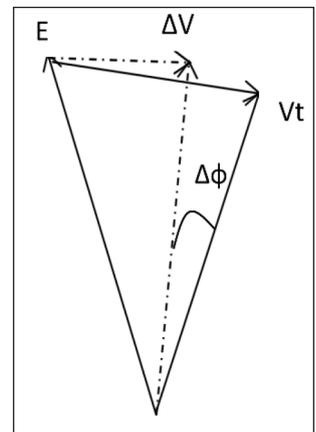
Fig. 7: Change of angle after loss of grid
